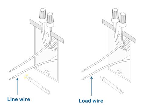
2) Turn off the circuit breaker. Label the Line and Load wires.
